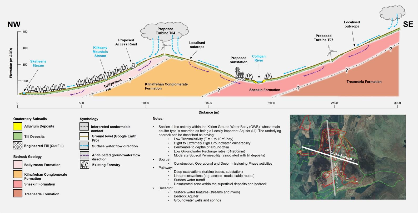
Figure 11.3: Conceptual Site Model (CSM) – NW-SE Cross-Section
